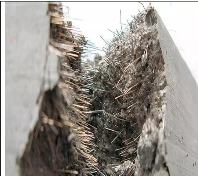
**Fiber** is a specialized additive for concrete and construction mixtures. The addition of fibers to a concrete mix substantially improves its performance characteristics, including tensile and flexural strength, crack resistance, abrasion resistance, impact resistance, ductility, and more. Basalt fiber can be incorporated into any type of concrete —decorative and standard, heavy-weight, aerated, foam concrete, and others. It is used in the production of:
