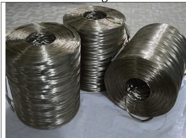
Basalt roving is produced by the way of melting basalt rock in a furnace, producing fusion through bushing assembly, funneling incessant fibers into a filament yarn, applying lubricating agent, winding filament yarn, drying filament yarn packages, filament yarn torsion into roving
