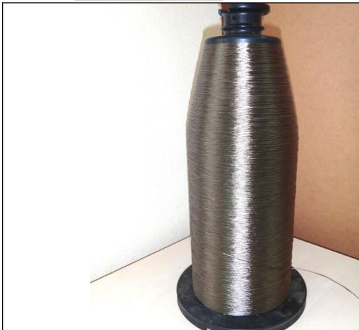
Basalt fiber is a product made by melting basalt rock and forming it into thin strands. The material is non-combustible, chemically inert, and resistant to ultraviolet light—unlike most modern materials. Fabrics made from basalt fibers are widely used in construction, automotive, and shipbuilding industries. They are employed as reinforcing mesh, protective screens, and fireproof barriers. Basalt-based material is also used for specialized protective clothing.
